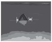
Figure 2-3 White Hot Thermal Display
