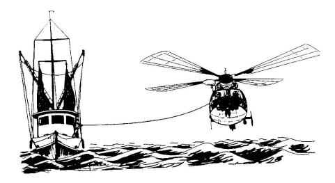
Figure 6-13 Indirect Delivery of Pump
