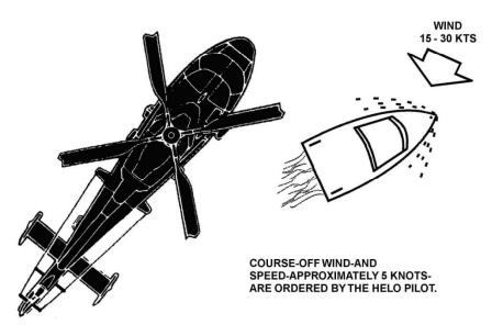
Figure 6-9 Helicopter-Boat Hoist
