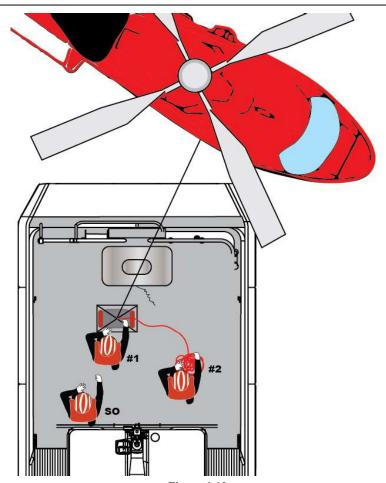
Figure 6-10 Overhead View of Deck Personnel, with M/J Basket and Trail Line
