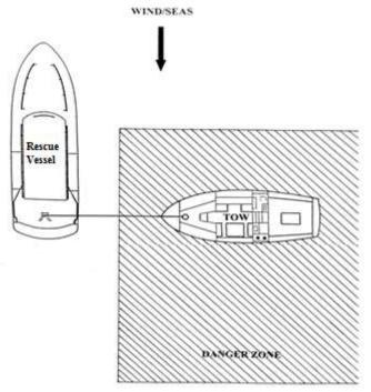
Figure 3-12 Optimum Position for Passing the Tow Rig
