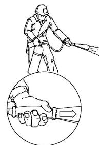
HOLD HORN BY INSULATED HANDLE... SQUEEZE TRIGGER
