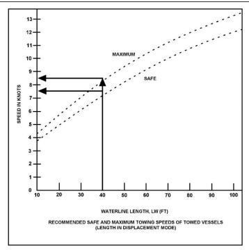
Figure 3-16 Calculated Safe Towing Speeds
