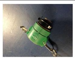
Figure 5-18 **Color-Coded Coupling**
